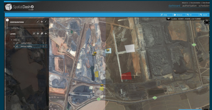
Figure 6 - The SpatialDash view shows the designated areas that a vehicle is allowed to collect material in green, dangerous areas in yellow and prohibited areas shown in red.
